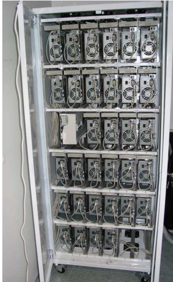
A 32 node AMD Athlon XP Mosix ATX blade server.
