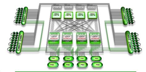
4Gb/sec end-to-end internal architecture including front end, disks, and back end
