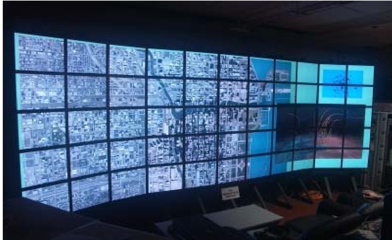
A "LambdaVision" display, built from 55 LCD screens. Total resolution: 17.600 x 6.000 pixels
