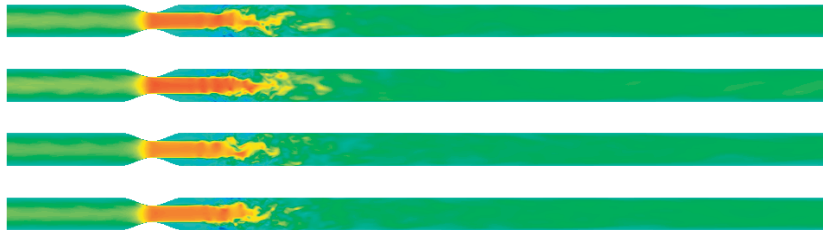
Figure 1: Instantaneous axial-velocity for four different time steps reveals a fluctuating flow in a post-stenotic region.
